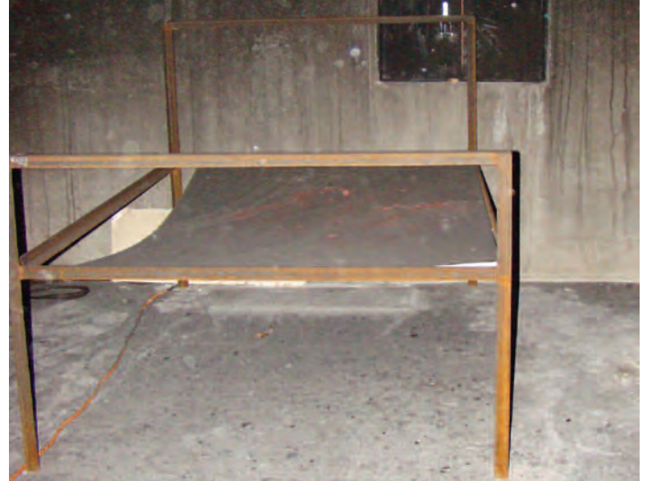
Figure 5: Noncombustible Furniture Used in the Time-to-Task Experiments
