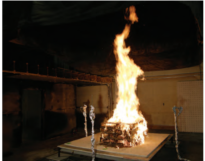
Figure 2: Test Burn of Pallets in Laboratory
